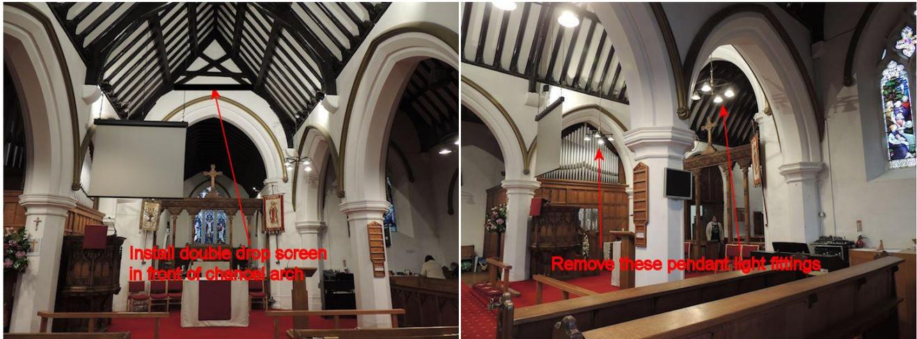
7. There are a pair of pendant light fittings which would through too much light on the screen, therefore it is recommended that these fittings are removed and the other light fittings are adjusted to illuminate the nave altar platform and high level chancel arch. **The DAC stated that the pendant light fittings should be carefully packed and stored for potential re-installation at a future date.**
